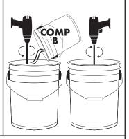
**4.** NOTE: In hot weather conditions, water can be added after initial mixing to adjust application consistency: max. 10 fl.oz. (0.3 L) per 46 lb (21 kg) unit Max. 16 fl. oz. (0.5 L) per 77lb (35 kg) unit. Add water and mix for an additional 1 - 2 minutes.
