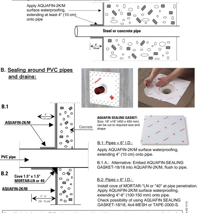
Note: Mechanically roughen PVC surface and degrease/clean with isopropanol or acetone prior to application of AQUAFIN-2K/M.
