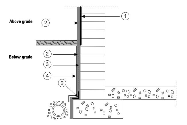
Seal exterior cracks, vertical and horizontal joints with AQUAFIN JOINT SEALING TAPE-2000 or CRACK SEALING TAPE.
