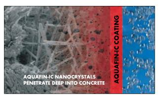
thereby blocking the passage of water. This reaction will continue to take place anytime water is present for the life of the concrete structure where by making the AQUAFIN-IC a truly permanent and integral waterproofing solution. The AQUAFIN-IC nano-crystals will also grow in and along static hairline crack sealing them and preventing further incoming water.
