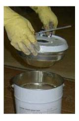
3. Completely drain Part B (hardener) into Part A (resin).
