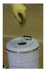
2. Pierce a hole through the top (rubber membrane) and the bottom of Part B.
